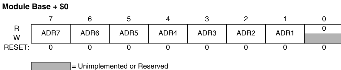
Figure 10-2. IIC Bus Address Register (IBAD)
