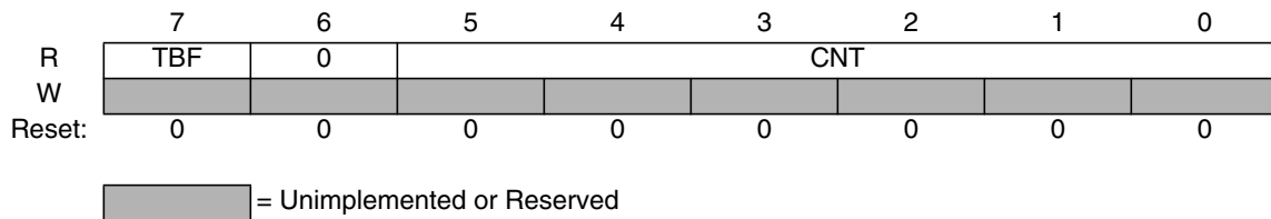
Figure 18-6. Debug Count Register (DBGCNT)
