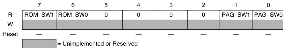
Figure 16-9. Memory Size Register 1
